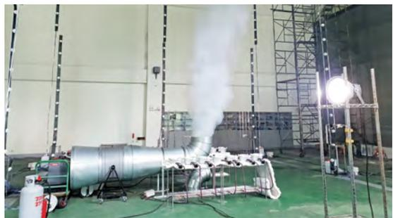
The ABRI developed hot smoke emission equipment and provides on-site hot smoke test verification
